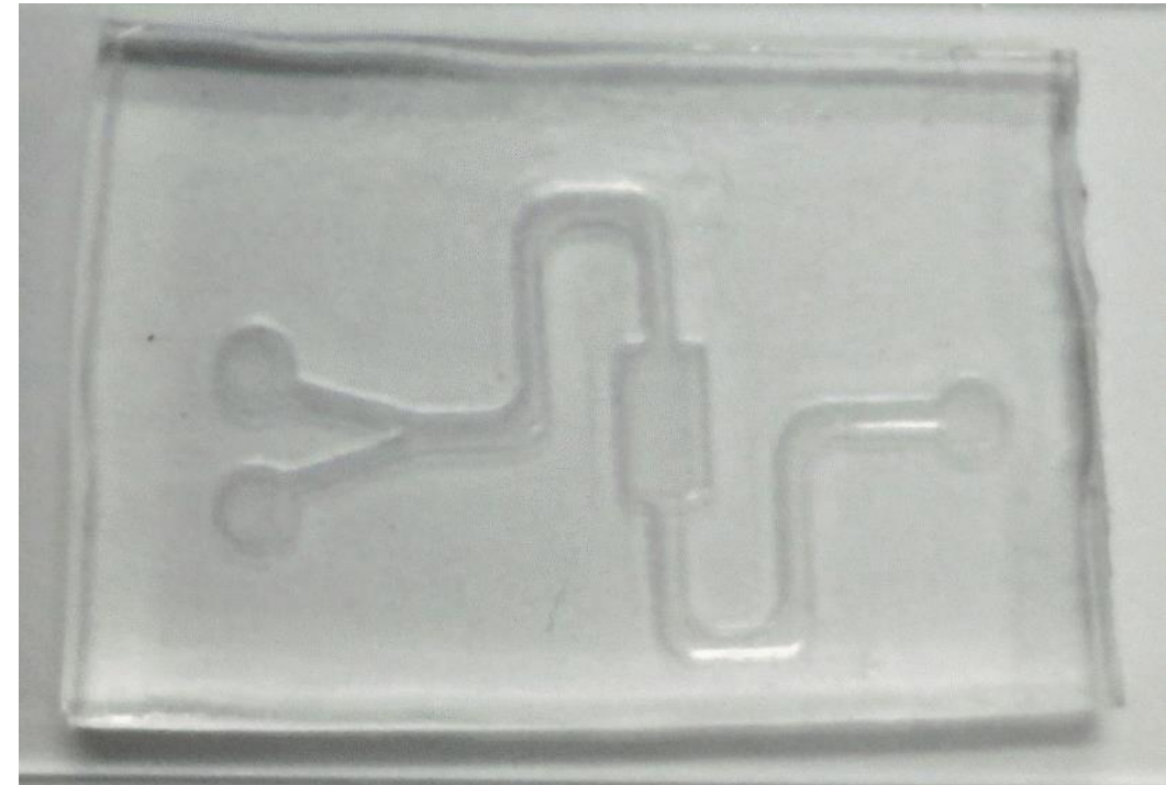
SU-8 molding of PDMS for microfluidic devices [2]
